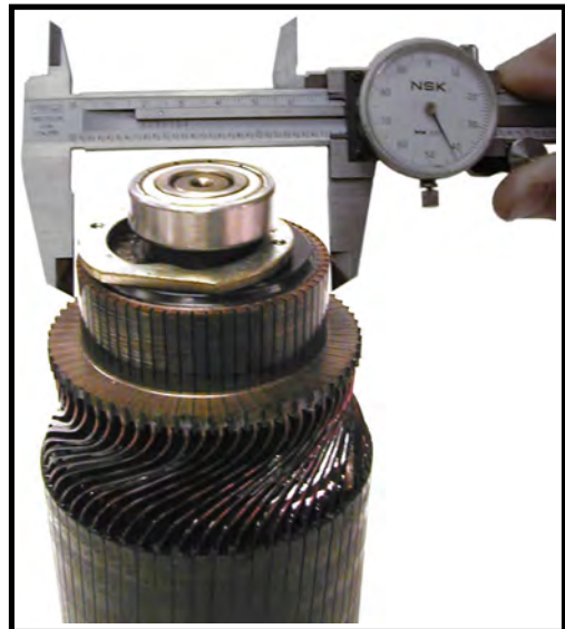
Example of freshly cut commutator
